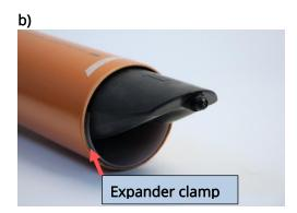
**b)** Push the valve into the pipe until at least the expander clamp is completely in the pipe.
