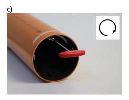
c) Tighten the screw in direction of the arrow with the original tool. To guarantee an optimal functioning the bolt has to be centred in the upper part of the pipe.
