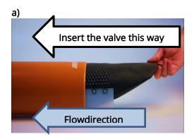
a) Before installation, completely loosen the clamping mechanism and moisten the valve surface with water. (Possibly soap water)
